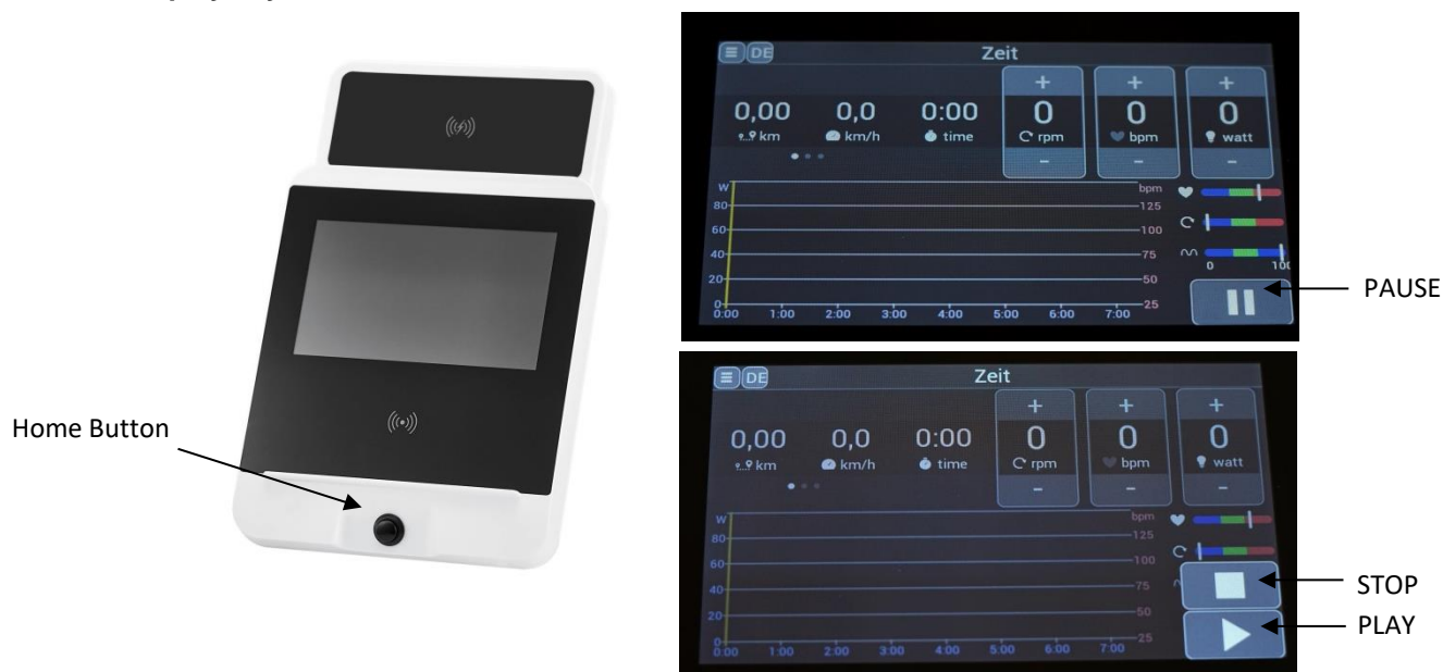
Fig. 2: Monitor view, explaining the button functions, actual view may vary in colour, button assignment is the same.
