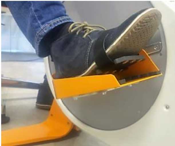
Image 33: Release of the foot rest in case the magnetic force is exceeded (> 70N)
