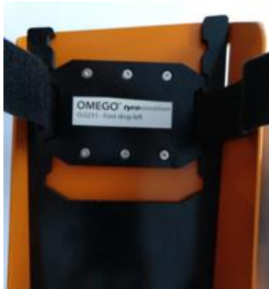
Image 13: Foot fixation with magnetic coupling
