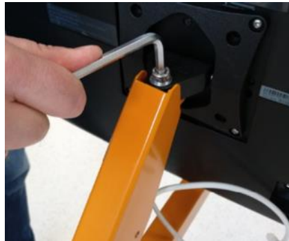
Image 24: Secure the All-IN-ONE PC with a screw on the monitor arm
