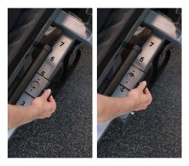
A second way to adjust the length of the drive belt is to pull the drive belt further out through the belt stop. This could be useful in rehab when you want to restrict the extension of the knee joint.
