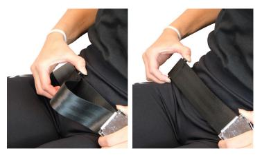
To lock the belt, put the flat part in the buckle. To release, lift the flap of the buckle and pull out the flat part. If you do not intend to use the seat belt, place it behind the backrest and lock it together.
