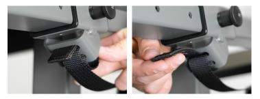
When you are happy with the new length of the drive belt, tighten any slack in the belt by pulling at the magnetic end before reattaching it to the beam.
