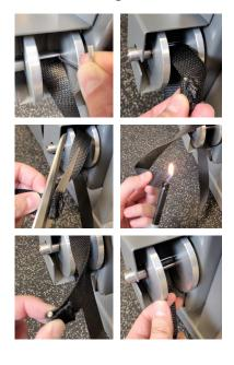
If damage to the drive belt occurs close to the shaft it is possible to cut off the damaged end and reattach the new end.
