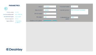
The sleep mode delay time (20 minutes by default) is adjustable from the scroll-down menu, allowing the administrator user chose the inactive time before the screen turns off. The device won't go on sleep mode during a session.
