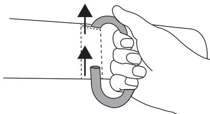
If both handles are on the device, first remove the handle on the side where the hook-and-loop fastener is located.
