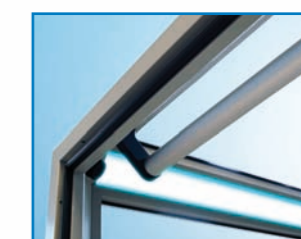
Fixed exit assist handle and LED lighting located in the cabin ceiling
