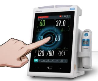
The 8-inch capacitive touch screen monitor, featuring in its ultra-narrow bezel design, quick-responding touch sensitivity, satisfies end users' clinical needs of simple operation and clear display of vital sign measurements.  Open to a variety of mounting solutions, both wall mount and movable trolleys for option
