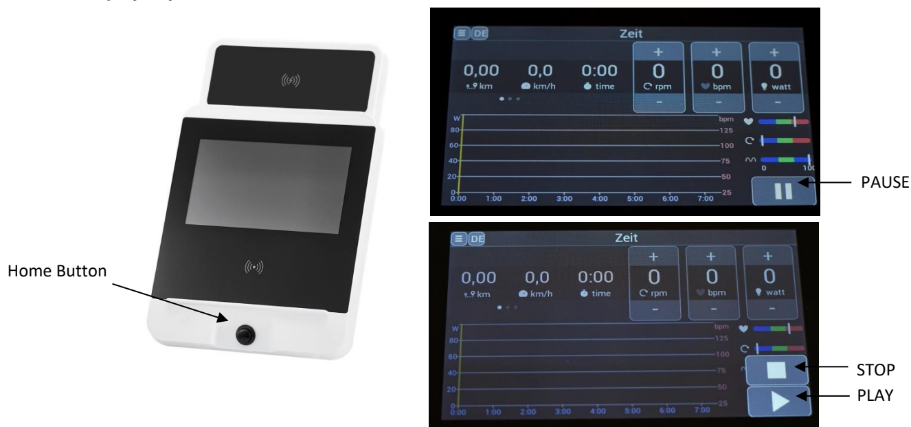
Fig. 9: Monitor view, explaining the button functions, actual view may vary in colour, button assignment is the same.
