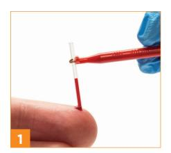
Collect 20  $\mu$ l blood sample in capillary.
