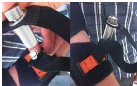
Illustration 13: You may only then close the magnet coupling by joining both magnetic parts to each other.
