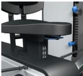
The starting position can be adjusted to several different levels with the grab handles located on both sides of the release lever. When exercising make sure that, the cervical spine remains in the neutral position and the head is not moved forward.
