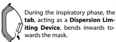
During the inspiratory phase, the **tab**, acting as a **Dispersion Limiting Device**, bends inwards towards the mask.
